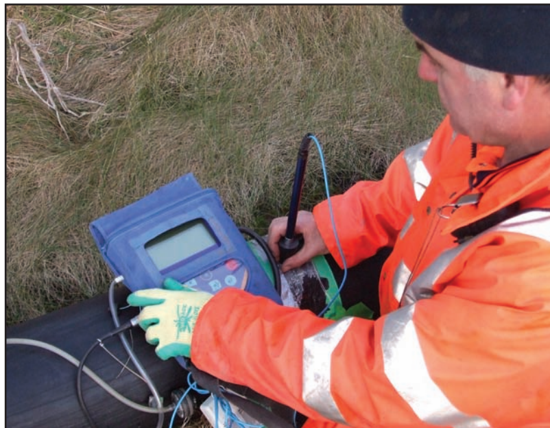
A GA2000 portable landfill gas analyser is used to check gas quality, pressure and flow
